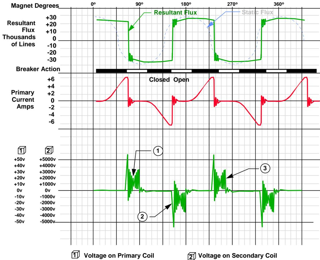
**Figure 14. Waveform Representation when Firing a Spark Plug in Engine Cylinder**
