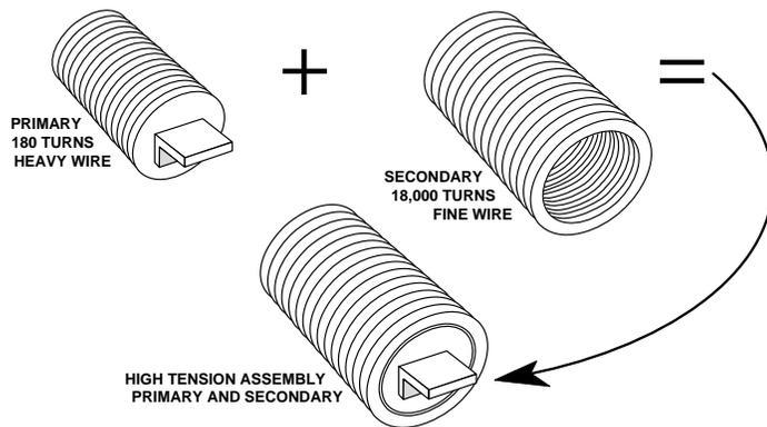
**Figure 13. Evolution of Coil for High Tension Magneto**
