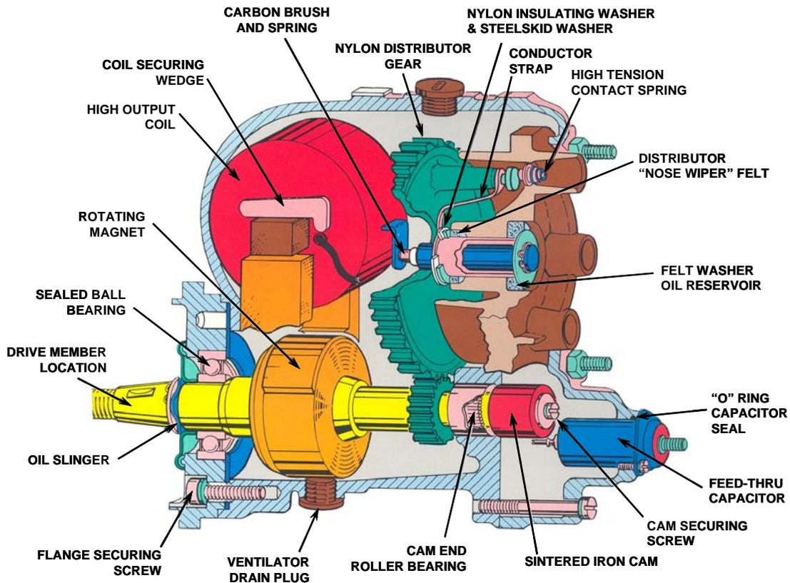
**Figure 16. The TCM S-1200 Series Magneto Cutaway Diagram**
