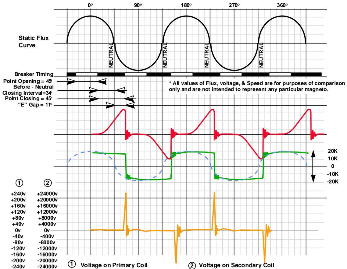
Figure 12. Operating Circuit Waveforms of a Magneto
