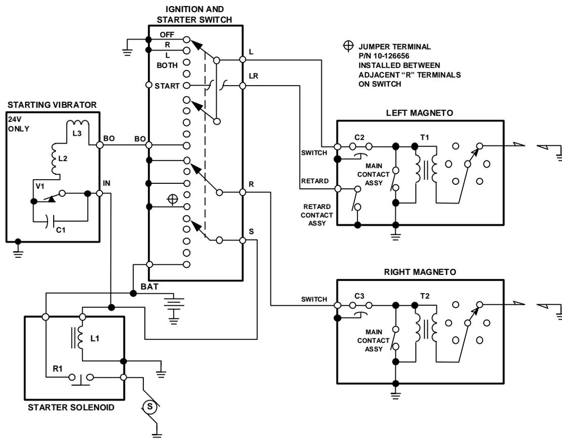
**Figure 15. Schematic Diagram of Magneto Circuit and Starting Vibrator**
