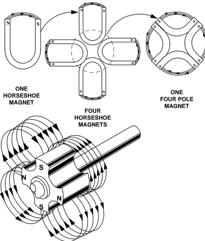
Figure 7. Four Pole Rotating Magnet
