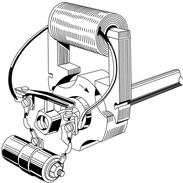
**Figure 11. Breaker Points and Condenser to Interrupt Primary Current**
