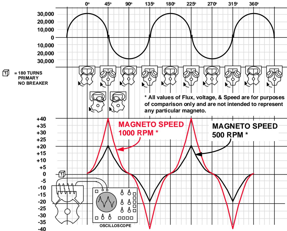
**Figure 10. Static Flux Curve and Voltages Generated by Rotating Four Pole Magneto**
